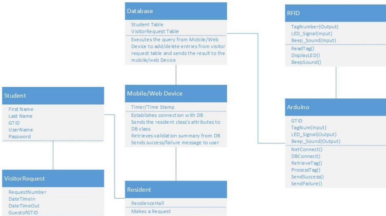
The object diagram for the software module is below:
