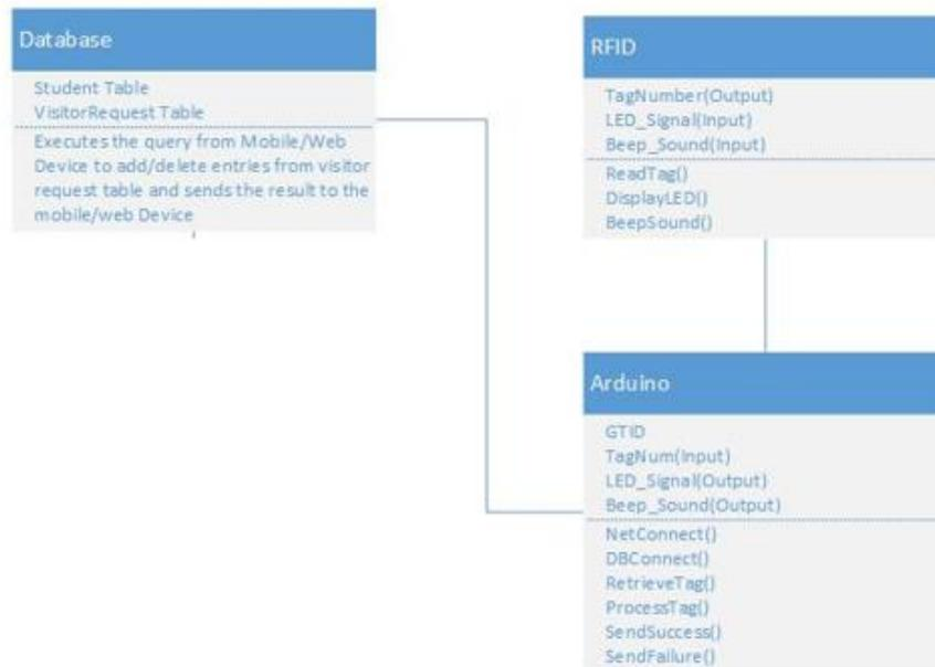
The class diagram for the entire system is below:
