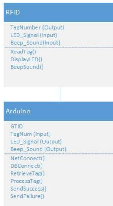
The object diagram for the entire system is below:
