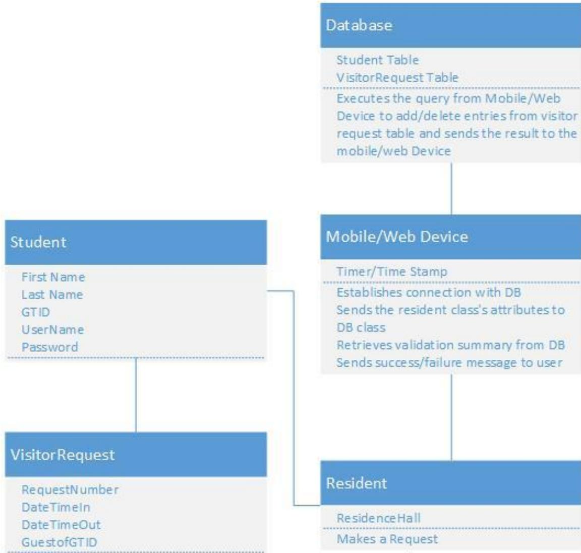
The class diagram for the hardware module is below:
