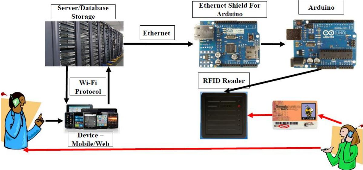
The secured entrance system for facilities has two main modules. The software module contains the database and the web application, whereas the hardware module contains the Arduino, its Ethernet shield and the RFID reader. The class diagrams for the software module is below:
